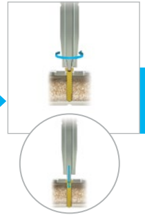
Lock 2.3 mm Hexalobe MultiScrew into Plate
