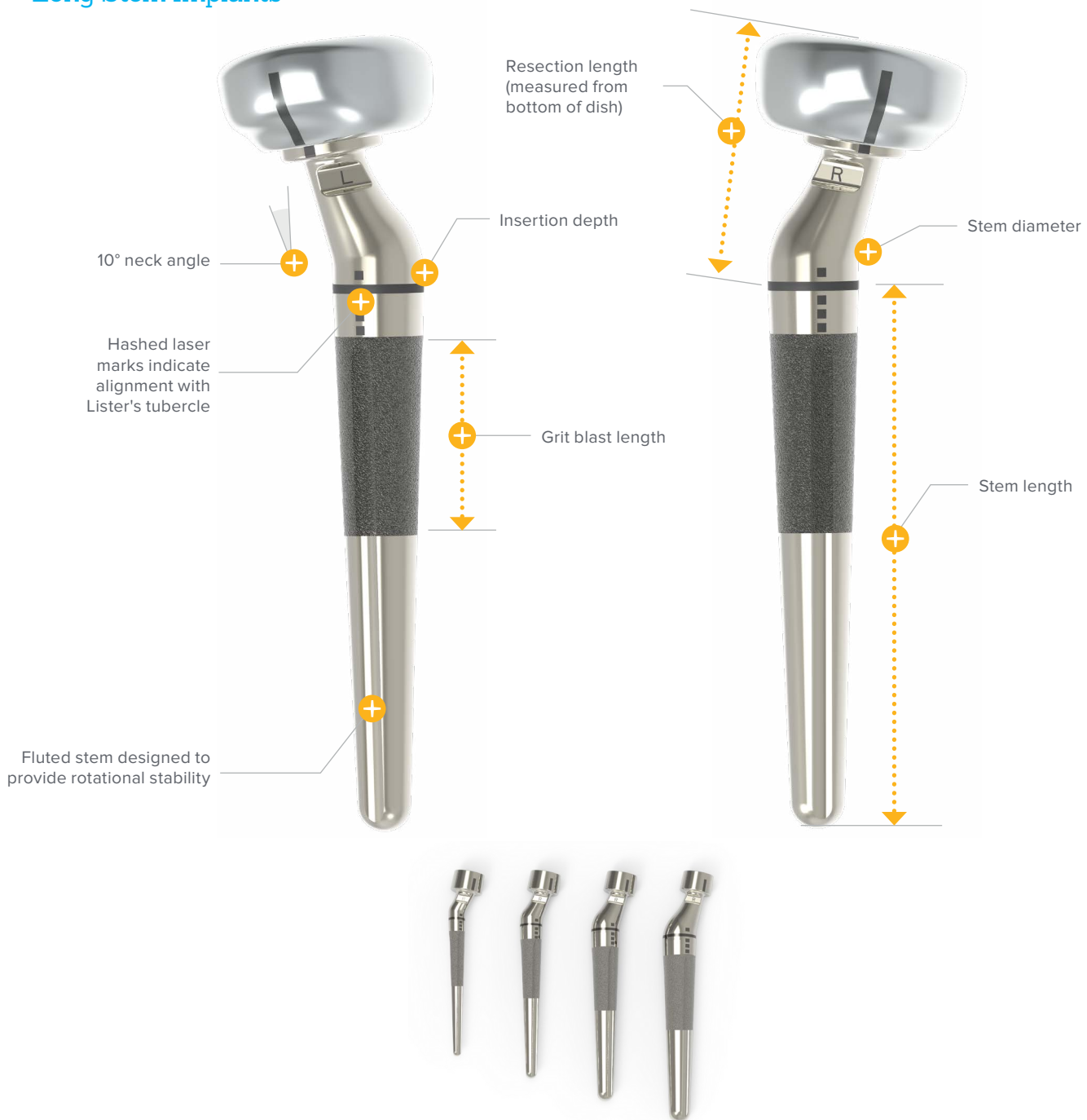
Long Stem Implants: 6–12 mm diameters, (2 mm increments) (TR-SLXX-S)
